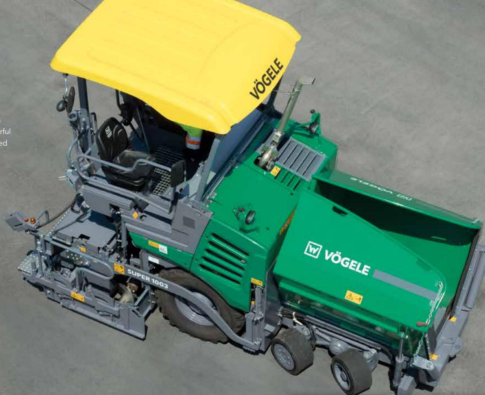
» **Rapid transport under its own power** at up to 20km/h - a feat the SUPER 1003 is optimally equipped for. The paver can optionally be equipped with a lighting system approved for use in traffic. As a result, this machine meets the basic requirement for driving on public roads.
