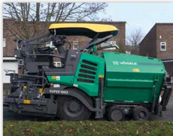
» **The slim paver design,** with no protruding edges and a compact overall length, makes it very easy to work and manoeuvre on tight job sites.
