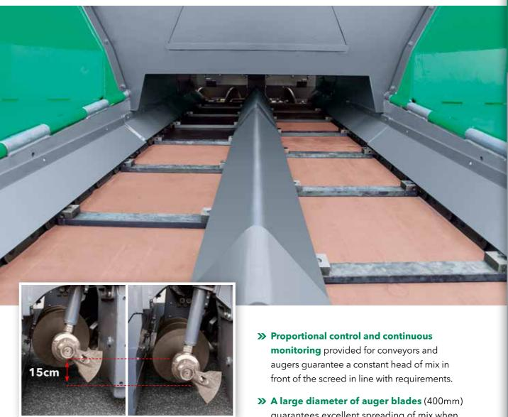
The height of the auger complete with bearing boxes and limiting plates for the auger tunnel can be hydraulically adjusted by up to 15cm across the full pave width. This optimizes the head of mix in front of the screed, even when paving thin layers or when layer thickness varies.
