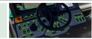
The paver operator's console is extremely clear and has been designed according to practical principles. All functions are combined into logical groups, so that the operator finds each function exactly where he would expect it to be. On the ErgoPlus 3 console, all push-buttons are easily identifiable by touch even when wearing work gloves.
