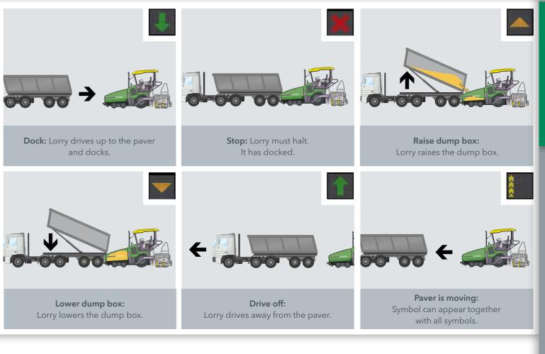
The core element of the PaveDock Assistant are the signal lights on the paver and the associated control elements on the paver operator's ErgoPlus 3 console.
