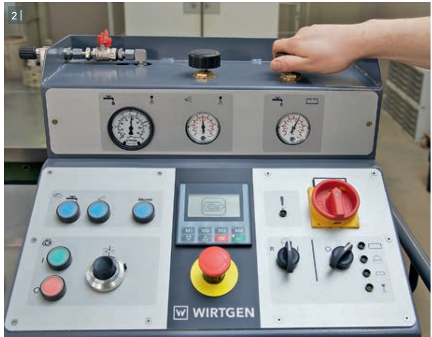
2 | The clearly and logically structured control panel permits easy setting and monitoring of important parameters.
