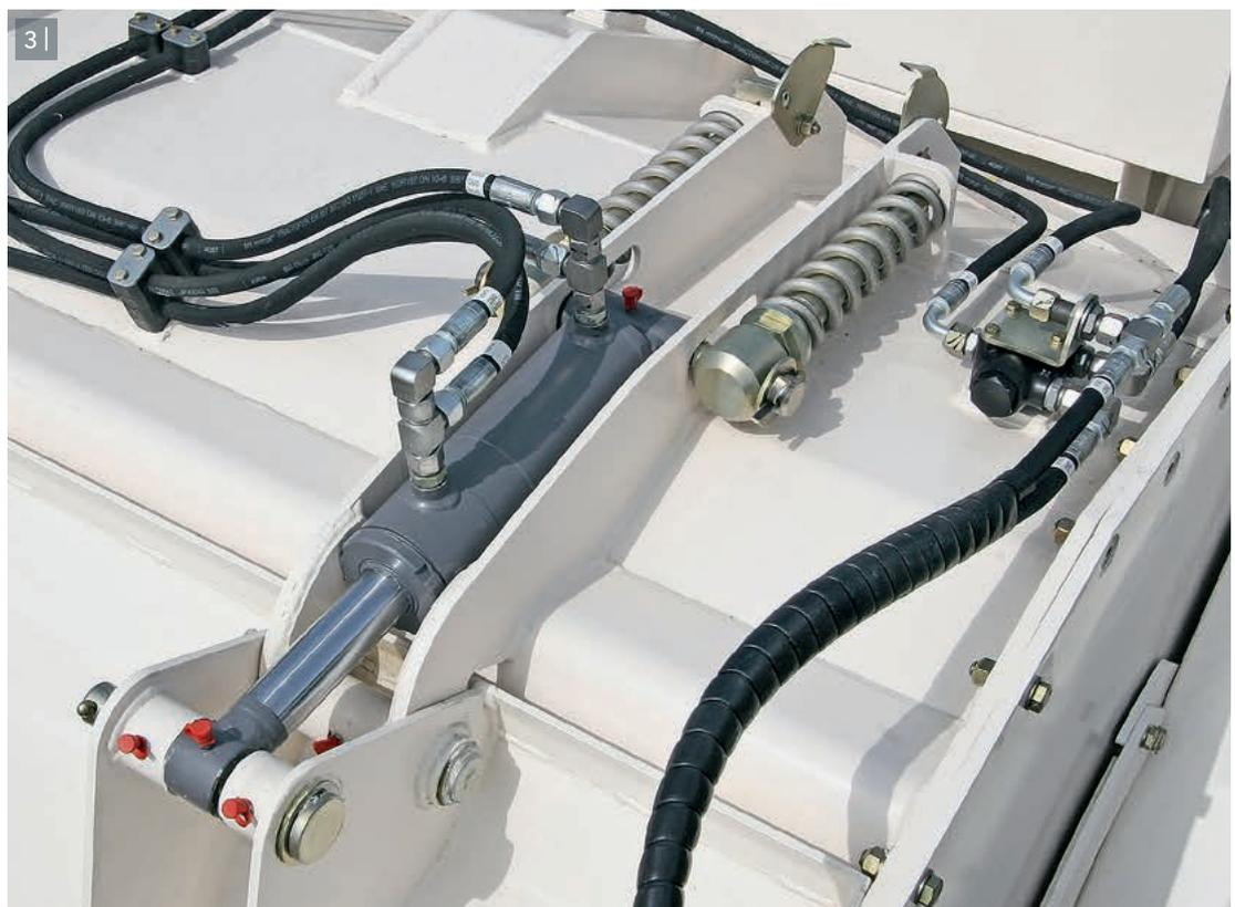
3 | Long spring assemblies ensure optimum contact pressure of the rotor plate.
