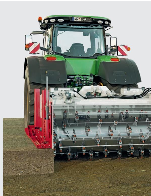
2 | Combined with a mechanical retainer, the side plates guarantee a consistent working depth.
