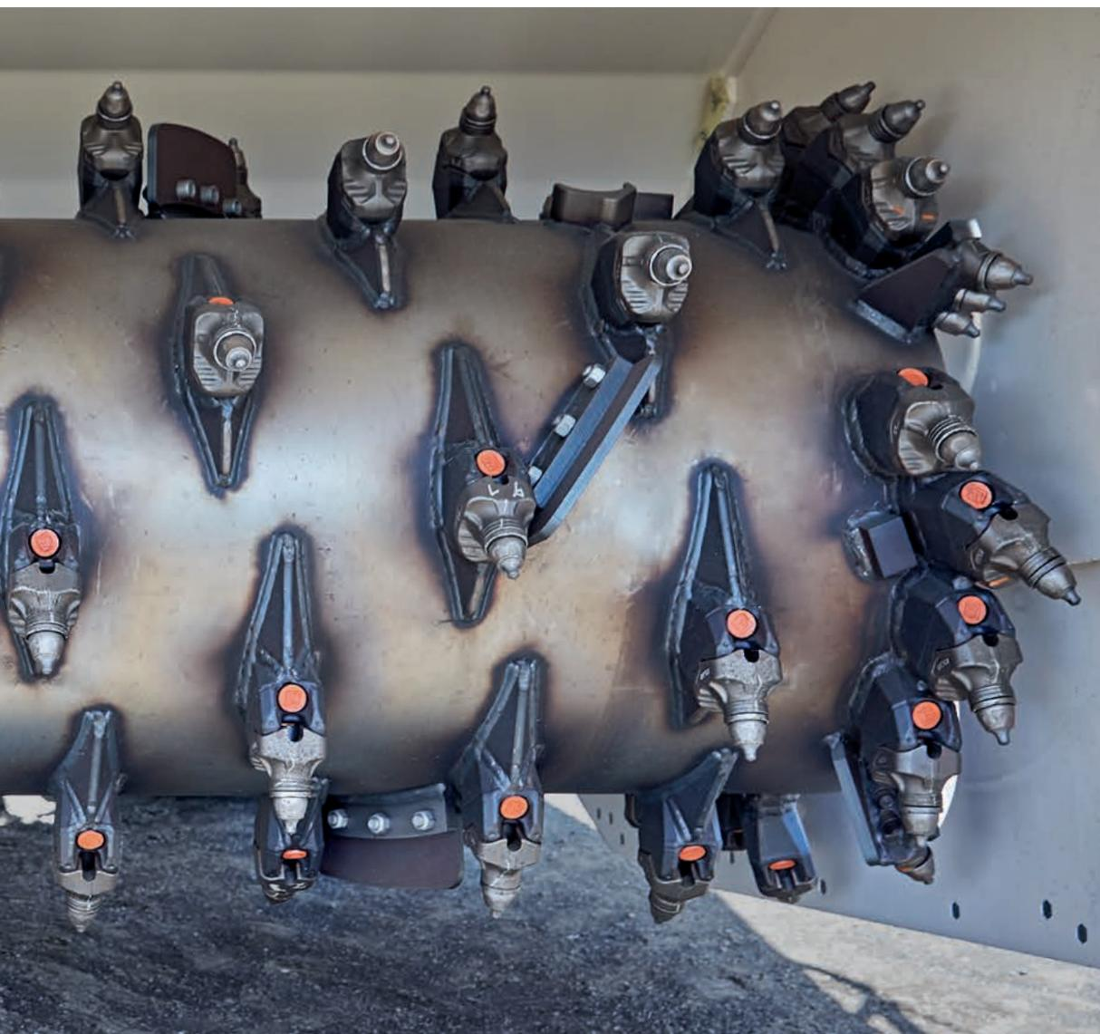
2 | The quick-change toolholder system HT22 significantly reduces operating costs of the machine.
