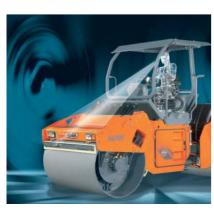
070V ASC - Articulated tandem roller with vibratory and oscillating drum
