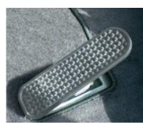
Hydraulic slewing brake pedal is standard
