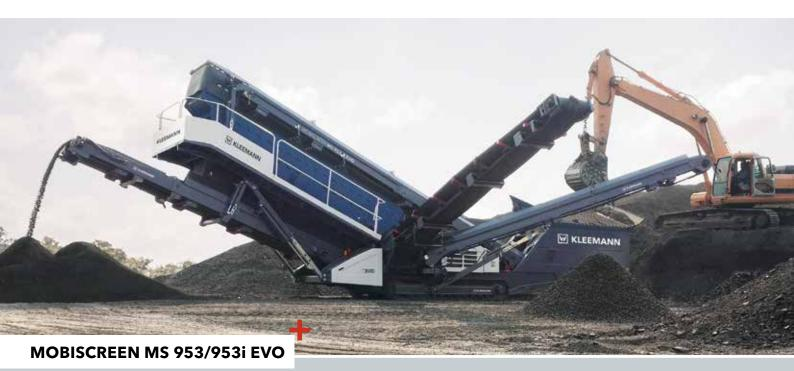
The mobile screening plant MOBISCREEN MS 953 EVO is equipped with a 9.5 m<sup>2</sup> screen box. The triple-deck screening plant impresses with a feed capacity of up to 500 t/h. It is operated by a modern control system. All functions are thus easy to control, operating statuses and machine functions can be viewed at any time.
