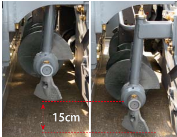
The augers of the SUPER 2100-2 are infinitely variable in height up to 15cm while paving.
