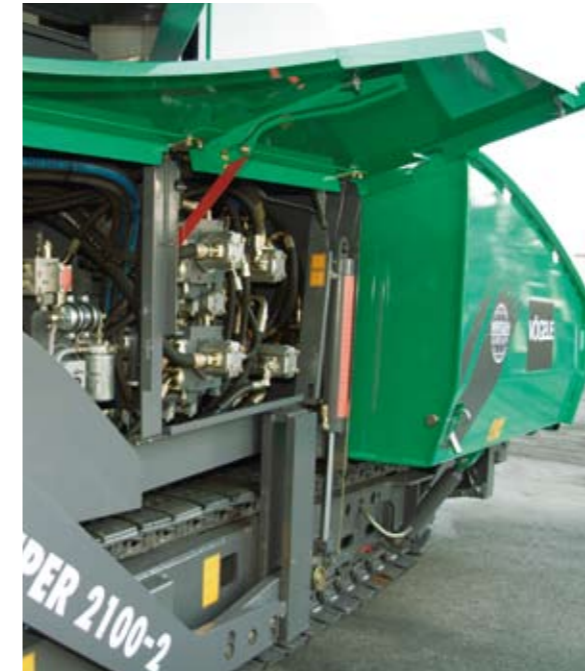
The standardized service concept conceived for the "dash 2" pavers means that servicing is quick and uncomplicated. Large hinged panels provide convenient access to all service points on the machine.
